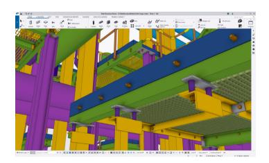
Tekla models contain everything needed for fabrication and construction, including welds.
